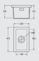
PLEASE NOTE: A DXF is not available, sink should be used as template. When undermounting, a minimum gap of 4mm must be left between the sink and the worktop.
