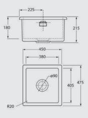
PLEASE NOTE: A DXF is not available, sink should be used as template. When undermounting, a minimum gap of 4mm must be left between the sink and the worktop.
