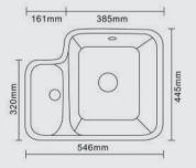
PLEASE NOTE: A DXF is not available, sink should be used as template. When installing, a minimum gap of 4mm must be left between the sink and the worktop.
